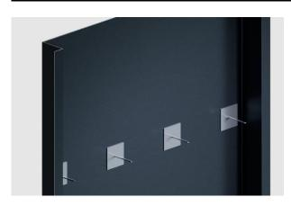
Install self-adhesive insulation pins on the inside of the cassette panel. Make sure they sit along the cavity barrier line.
