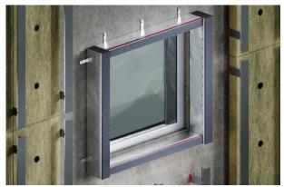
Around windows, vertical non-ventilated barriers should be installed on both sides, extending above and below the opening.
