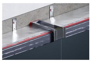
The CFS-NVB piece should extend 20mm above and below the ventilated barriers.
