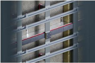
In a two-layer system, when the façade vertical rail partially intersects the leading edge of the barrier, attach a section of CFS-NVB in front of the rail to ensure no gap between the rail and the panel.
