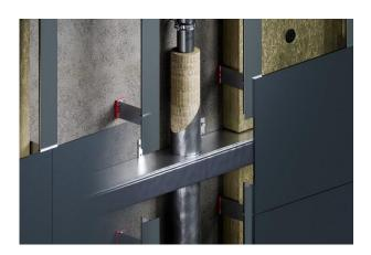
Install 25 mm thick locally sustained mineral wool insulation around the metal pipe, so that the insulation extends 300mm above and 400mm below the barrier.
