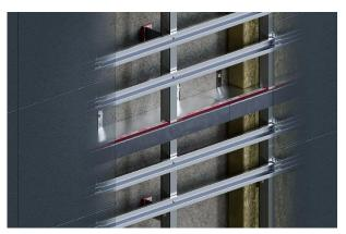
When the façade vertical rail fully intersects the cavity barrier, notch the barrier to accommodate the rail and ensure no gaps.
