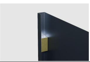
Cut two sections of CFS-NVB to be tight fit to the edge return of the panel.
