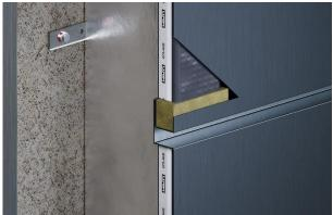
Cut a section of CFS-NVB matching the barrier thickness and friction fit it into the cassette panel return, ensuring no gaps.
