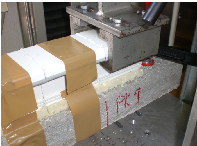
Fig. 7 Test set-up for tensile test
