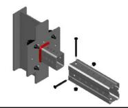
3. Beam Clamps - per analytical Calculation
