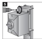
Tighten using a screwdriver with torque clutch or Hilti torque tool X-BT  $\frac{1}{4}$ " - 20 Nm [14.8 ft-lb] T ≤ 20 Nm (≤ 14.8 ft-lb)
