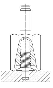
The stainless standoff adapters M8-MR 50, M8-MR 75, M8-MR 100, M10-MR 50, M10-MR 75, M10-MR 100, W10-MR 50, W10-MR 75 and W10-MR 100 may also be used in combination with X-BT-ER fasteners for electrical applications.
