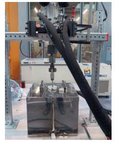
The chamber is heated as long, till the test temperature of the steel base material is reached. The right photo shows the temperature sensor ("black wire") which is fixed in the base material in a small bore hole of 2 mm diameter close to the X-BT threaded fastener. If the target temperature in the base steel is reached, the tension pullout test is performed (with closed chamber). The photos show the opened chamber after the tension test was executed.
