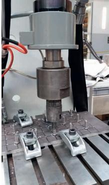
Dynamic tension loading on the new generation X-BT threaded fastener demonstrates excellent robustness of anchorage.
