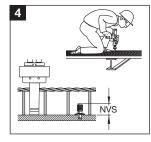
Drive fastener with BX 3-BTG tool or DX 351 BT G tool and 6.8/11 M brown cartridge.
