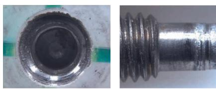
Drilled holes after 480 hours of salt spray test and after pull-out of the X-BT fasteners. These holes appear clean and no evidence of corrosion is visible.
