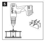
Tighten X-FCM-R (HL) with 5 mm Allen-type bit.
