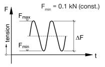
Principle sketch of cyclic tension tests
