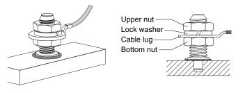
Double point connection for all X-BT-ER M8/7 SN8, X-BT-ER M10/7 SN 8, X-BT-ER W10/7 SN 8
