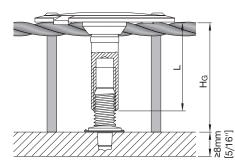
Thickness t of disc of X-FCM-R fasteners: X-FCM-R HL: t = 1.5 mm X-FCM-R: t = 1.25 mm
