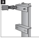
Drive X-BT fasteners with **BX 3-BT** tool or **DX 351 BT** tool and 6.8/11 M brown cartridge.
