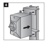
Position unit on studs and hold in place. Fit washers and start tightening by hand to avoid cross threading.
