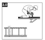
Pre-drill with **TX-BT 4.7/7** step shank drill bit.
