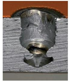
Steel base material after 10 years of exposure to sea water and pull-out of the X-BT fastener. The hole appears clean and no evidence of corrosion is visible. If the surface of the less "noble" material (1) is greater than that of the more "noble" material (2), it will act as a very small cathode and the current density on the "large anodic" less noble material will be very small. Further, this also implies a very low rate of corrosion of the "less noble" material due to electrochemical effects.
