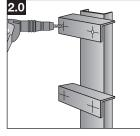
Pre-drill with **TX-BT 4.7/7** step shank drill bit.
