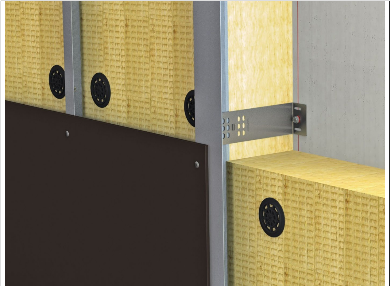
Figure 3 Typical vertical rail/bracket arrangement
